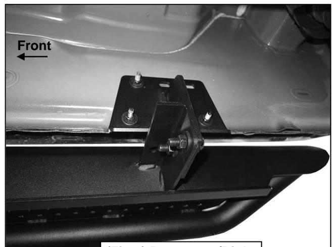
(Fig 8) Passenger/Right Rear Sidebar installed
